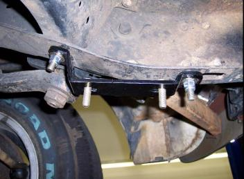
You can now fully tighten the frame bolts at this time.
