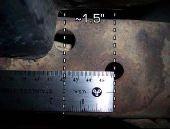
Go to the passenger side frame rail and measure the same dimension and mark the frame with a paint pen. Drill out the hole using a **7/16**" drill bit.
