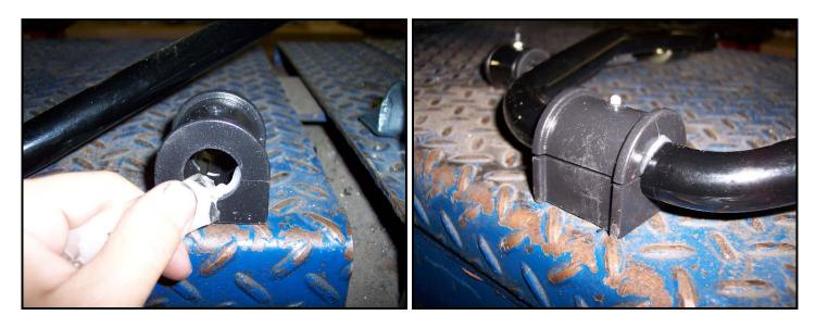
Slide the bushing brackets onto the bushings as shown below.
