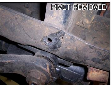
Once the holes are clear, grab the 3/8" x 1.5" hex bolts & washers from the "front" hardware bag and insert them into the rivet holes facing down.
