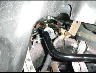
14) Reattach the endlinks to the sway bar in the same manner as removal. Fully tighten all hardware
