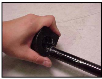
13) Feed your new Hotchkis sway bar into the sway bar location in the same manner as removal. Make sure the bar is oriented as shown in the picture. Place the provided bushings mounts over the bushings and make sure the 90° zerk fittings are facing outboard. Fully tighten the stock bracket bolts.
