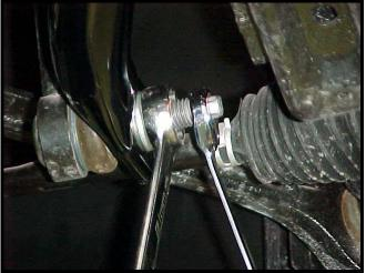
You are now finished with the front sway bar installation! Make sure that all hardware is fully tightened before driving the vehicle. Let's move on to the rear sway bar installation.
