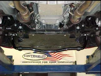
7) Install the subframe mounts back onto the vehicle. Fully tighten all hardware at this time (including the endlink bolts!)
