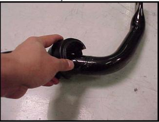
6) Reinstall in the same manner as removal. Attach the endlinks to the sway bar. Do not tighten at this time
