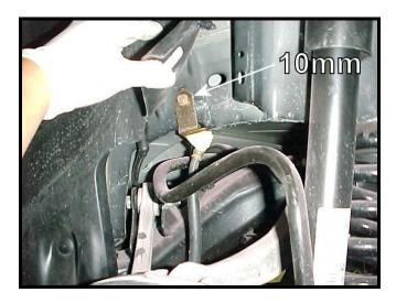
Next, you will need to drop the exhaust system for clearance. Unbolt the mid-brace removing the 4 bolts using a 13mm socket. Spray the rubber hangers in the picture with WD-40 and slide the rubber hanger off the exhaust support. Unbolt the remaining rear hangers using a 13mm socket. Be careful, for the exhaust will drop down once these bolts are out.
