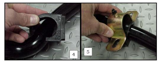
5R. After you determine there's enough clearance for the bar, note the approximate location of the sway bar axle bushings.
