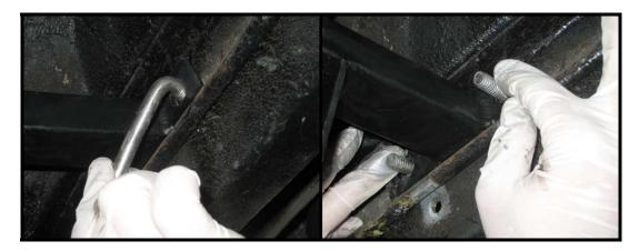
Place washers and nylock nuts on the U-Bolt. Tighten one side of the U-Bolt partially, and then tighten the other side of the U-Bolt partially alternating back and forth until fully tightened to guarantee the bolt is tightened properly.
