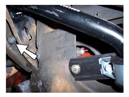
c) Loosen and remove the nut connecting the strut rod to the lower control arm.
