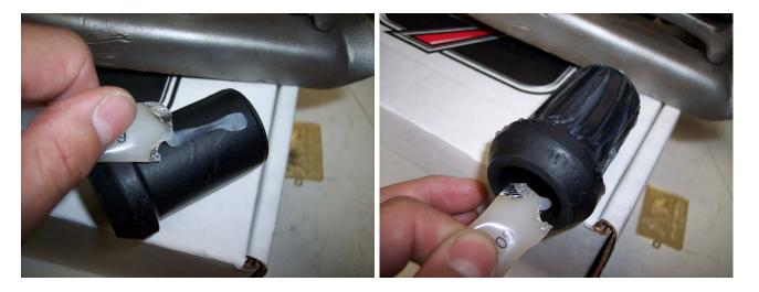
Insert the bushing into the outer sleeve by itself. Then insert the pin and inner sleeve into the bushing. The assembly is now complete.
