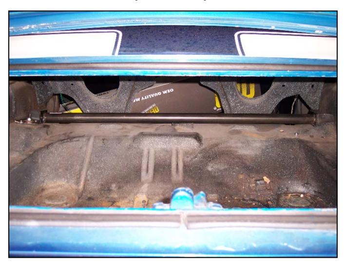
4. Install the supplied washers and nuts onto the studs. Fully tighten all hardware. You are now finished with this installation.
