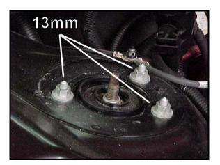
7) Once the shock is out of the car, mark the shock top hat and lower perch with whiteout or other marking tool. This will ensure proper orientation for reinstallation.
