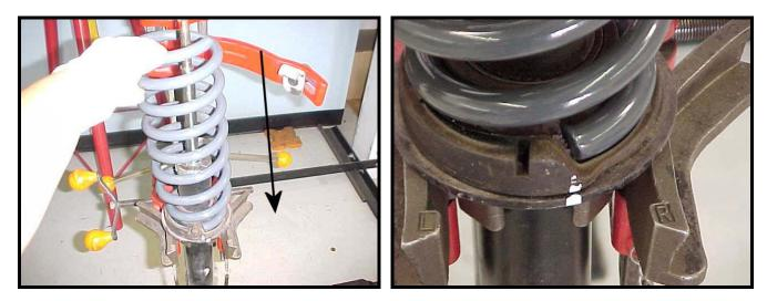
12) Before compressing the spring, test fit the top hat onto the shock shaft and see if your marks line up. If not, rotate the coil spring until they align.
