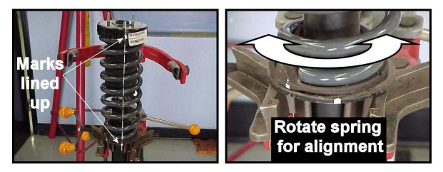
13) Once aligned, compress the coil spring and install the shaft nut back on. Fully tighten hardware.
