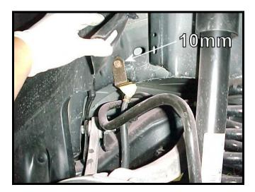
5) Next, you will need to drop the exhaust system for clearance. Unbolt the mid-brace removing the 4 bolts using a 13mm socket. Spray the rubber hangers in the picture with WD-40 and slide the rubber hanger off the exhaust support. Unbolt the remaining rear hangers using a 13mm socket. Be careful, for the exhaust will drop down once these bolts are out.
