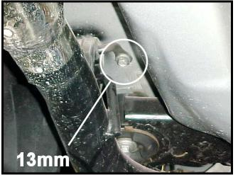
6) Support the rear axle pumpkin housing with a jack. Try to use wood or a rubber pad to cushion the contact point of the jack and housing. Remember the jack stands should still be supporting the rear of the vehicle.
