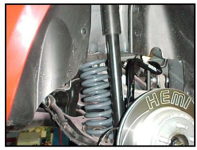
12) Once everything is in place, raise the rear axle into position. Do not raise all the way up! You will still need some wiggle room to line up the cradle bolt holes. Start each bolt by hand to ensure proper threading. Once thread started, fully tighten the cradle bolts using a 18mm socket. Torque bolts to 133 ft-lbs.
