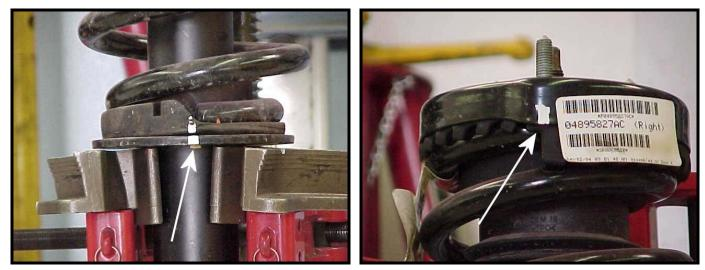
8) Secure the spring/shock assembly in your spring compressor and remove the shaft nut using a 18mm socket. Retain hardware for reinstallation.
