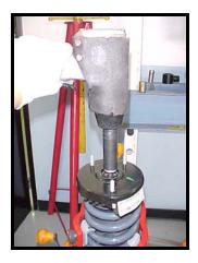
14) Reinstall the spring shock assembly in the same manner as removal. When installing the lower shock bolt make sure the hole lines up with the shock clevis. Make sure the threads start correctly by threading the bolt by hand. Once properly threaded fully tighten hardware.
