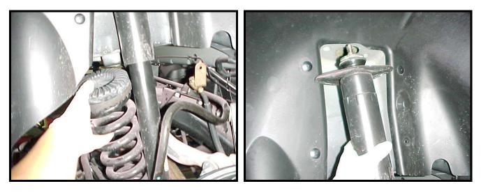
10) For each shock, unbolt the shaft nut using a 15mm socket. Remove the washer, top hat, and the boot to reveal the stock bumpstop. Replace the bumpstop with the provided Hotchkis polyurethane bumpstop in the same manner. Reassemble the shock. Fully tighten the shaft nut.
