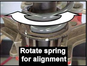
13) Once aligned, compress the coil spring and install the shaft nut back on. Fully tighten hardware.
