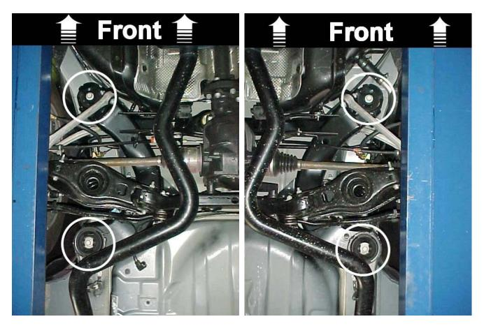
8) Lower the jack that supports the axle about 4-5 inches. Make sure not lower it too much to avoid damaging the rear brake hardline.
