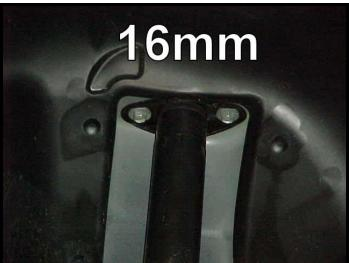
4) Pull back the plastic splash guard and remove the bolt that holds the brake line to the frame using a 10mm wrench or socket.
