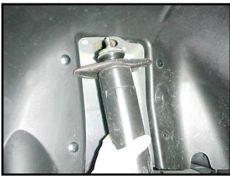
10) For each shock, unbolt the shaft nut using a 15mm socket. Remove the washer, top hat, and the boot to reveal the stock bumpstop. Replace the bumpstop with the provided Hotchkis polyurethane bumpstop in the same manner. Reassemble the shock. Fully tighten the shaft nut.
