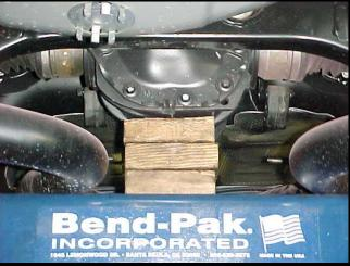
7) Once the axle is supported, you can unbolt the 4 bolts that secure the rear cradle to the frame using a 18mm socket.
