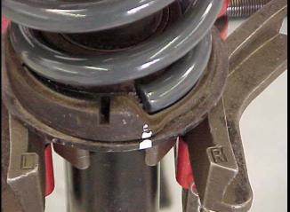
12) Before compressing the spring, test fit the top hat onto the shock shaft and see if your marks line up. If not, rotate the coil spring until they align.
