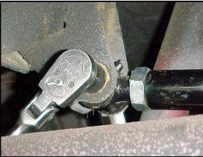
7) With the ends of the panhard rod secured, you can make any final adjustments to the length of the bar by loosening the jam nuts and rotating the center section. Extend the bar to move the axle to the right. Shorten the bar to move the axle to the left.
