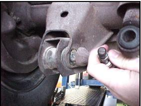
6) Use the grease provided to apply a heavy coat of grease to the bushings at both ends of the Hotchkis arm. Apply a light coat of grease to the bushing contact areas on the frame and axle.
