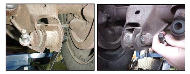
6) Use the grease provided to apply a heavy coat of grease to the bushings at both ends of the Hotchkis arm. Apply a light coat of grease to the bushing contact areas on the frame and axle.
