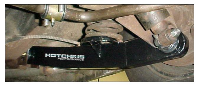
**IMPORTANT!** Check all hardware after the first five miles. For maintenance be sure to grease the bushings using the zerk fittings at least once a year (15,000 miles) or whenever excessive noise occurs. Use only a <u>non-lithium based grease</u>. Lithium based grease can wash out with water.
