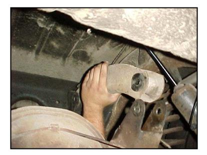
3) Check the stock arm mounting hole center-to-center measurement. The stock arm length should match the length of the Hotchkis upper arm center-to-center measurement.
