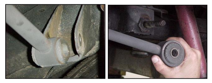
4) Match the Hotchkis panhard rod to the stock Chevy panhard rod. To adjust the Hotchkis panhard rod, loosen then jam nuts at each end. Rotate the middle section to shorten or lengthen the bar. DO NOT rotate the ends of the rod individually as this will affect the maximum and minimum adjustment of the bar.
