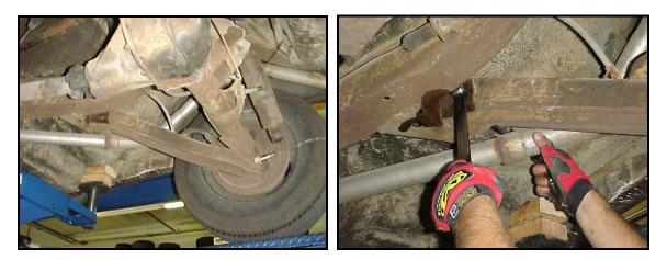
The hardware at the rear of the arm is easily accessed and should be removed. <u>Retain the stud for later</u> <u>use</u>. With all the hardware removed the stock arm should drop out of place.
