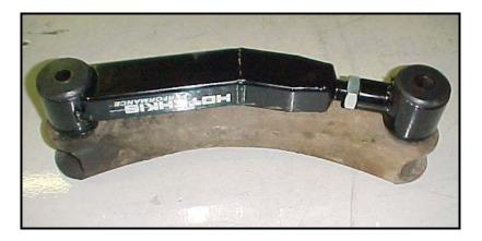
If the Hotchkis arm does not match the center-to-center length of the stock arm then you should adjust the length to match. Loosen the jam nut and rotate the head. Turn the head **clockwise to shorten** the length, and **counter-clockwise to extend** the arm. Hand-tighten the jam nut against the head to hold it in place for the installation.
