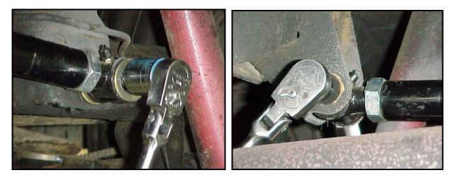
7) With the ends of the panhard rod secured, you can make any final adjustments to the length of the bar by loosening the jam nuts and rotating the center section. Extend the bar to move the axle to the right. Shorten the bar to move the axle to the left.
