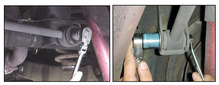
3) Remove the stock panhard rod. Rotate the top end of the bar out of the bracket on the frame and then pull the bar off the stud on the axle.
