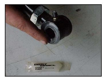
6) Install the Hotchkis panhard rod by sliding the thick 9/16" washer over the stud on the axle. Then slide one end of the bar over the stud on the axle and place the 5/8" washer on the end of the stud. Rotate the bar up into the bracket on the frame and use the new hardware. Torque the hardware at each end of the panhard rod to 30ft/lbs.
