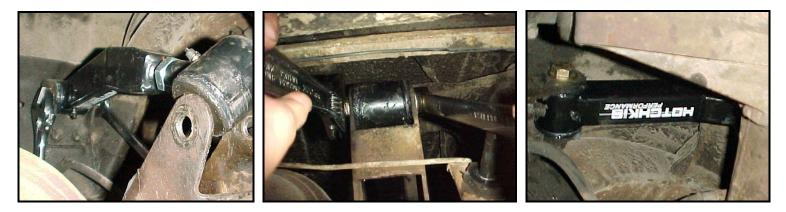
6) With the arm(s) in place, determine if any pinion angle adjustment is necessary. For stock vehicles no adjustment should be required. If the pinion angle needs to be adjusted downwards, the arm length needs to be shortened. If the angle needs to be adjusted upwards, the arm length should be extended.
