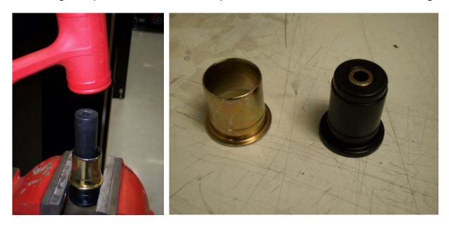
11. Normally with enough room, you can place the bushing can in the differential mount and hammer it in with a flat piece of wood. But, if there isn't enough room, then you will have to fabricate your own press tool. This is not as hard as it sounds.
