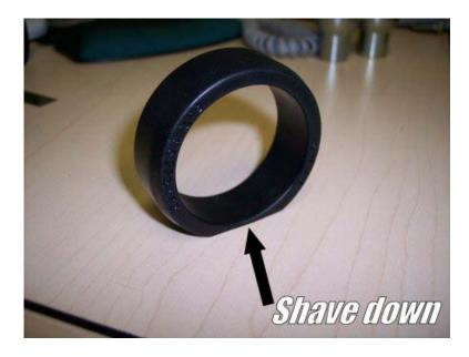
12. Once both cans are pressed in, lube the polyurethane bushings and push them into the can in the same manner. You may need to use a dead blow hammer or large channel locks to get the bushing in all the way.
