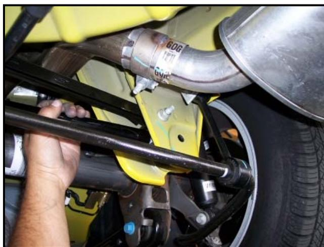
An adjustable panhard rod is used to give the owner the ability to laterally center the rear wheels with the chassis. This is usually needed with lowered vehicles.
