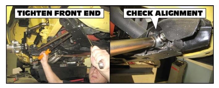
Restore torsion bar snap ring. Adjust the torsion bar tensioner back to where it was for proper pre-load.
