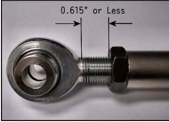
Center the heim joint so that it is not twisted one way or another. Tighten the heim joint jam nut.
