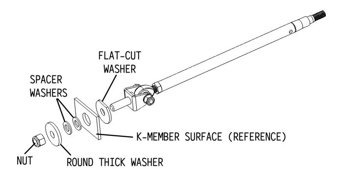
Install the large flat-cut washer onto the clevis stud and insert the front mount into the k-member hole.
