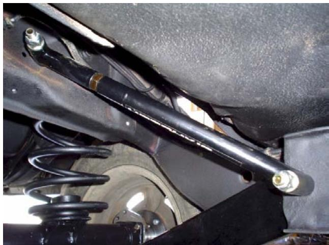
**NOTE:** For 78-88 models (part #1401) the curved section fits next to the lower trailing arm between the rear seat pan and the frame cross-member as shown in the photos below.
