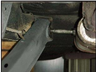
The hardware at the rear of the arm is easily accessed and should be removed. With all the hardware removed the stock arm should drop out of place.
