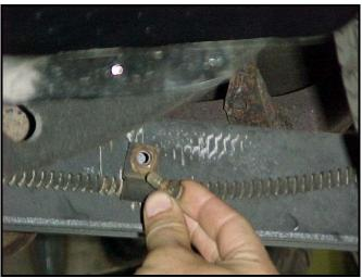
3) Unbolt the shock from the rear axle, and pull it clear of the mounting stud. Then remove the coil spring retainer plate from the trailing arm. **USE EXTREME CAUTION!** There will be **nothing holding the spring** to the trailing arm except the weight of the vehicle.
