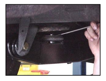
11) Reattach the brake line to the side of the Hotchkis arm using the tapped hole on the outside of the trailing arm. Use the new hardware provided.
