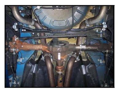
2. Disconnect the sway bar ends from both sides.
