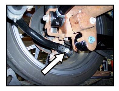
3. Disconnect the rear lower shock mounts on the both sides.
