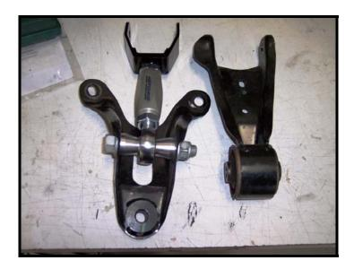
9. Install first the two (2) bolts from the upper mounts by having it finger tight, and then install the third bolt for the upper mount under the rear seat.
