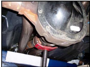
11. Reconnect the lower shock mounts and sway bar.
