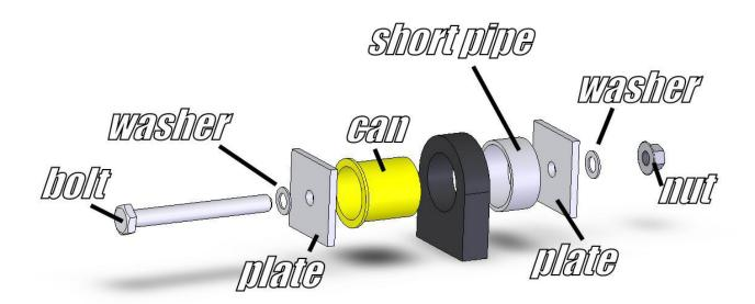
Use a ¾" wrench to hold the nut and a ¾" socket to tighten the bolt. The bolt may eventually run out of thread. When this occurs, you can replace the short pipe with the deep pipe.
