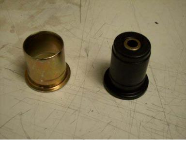
11. Normally with enough room, you can place the bushing can in the differential mount and hammer it in with a flat piece of wood. But, if there isn't enough room, then you will have to fabricate your own press tool. This is not as hard as it sounds.
