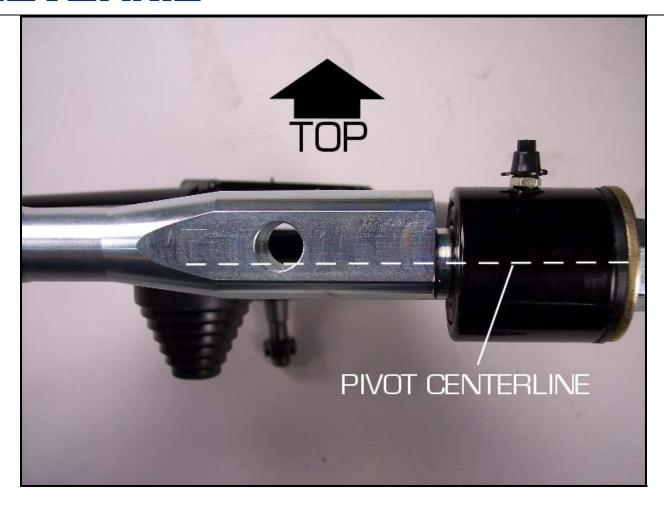
Install the cross shaft onto the vehicle first, using the same nuts that held in the stock arms.
