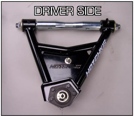
Please also note the orientation of the cross shaft. The a-arms are designed to have the inner pivot lower than the stock location. This improves the camber gained for better front grip.
