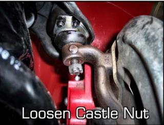
Smack the spindle mount to break loose the ball-joint stud from the spindle. The spindle should drop down and rest on the castle nut. Do not remove the castle nut yet!
