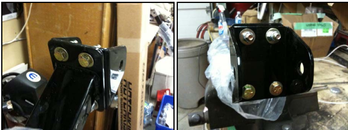
Mock-up shown with Hotchkis leaf spring mount
