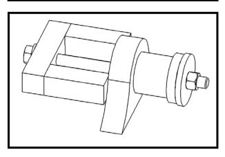
Step 2: Tighten the nut until the bushing is pressed securely into the mount. The bushing will not be pressed all the way to the flange due to the increase in diameter of the can. This is normal.
