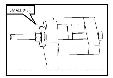
Step 4: Tighten the nut until the bushing is free to remove.
