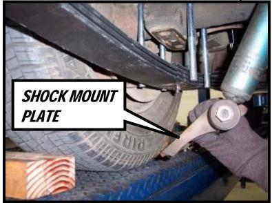
**5.** Loosen the two rear bracket nuts. *NOTE: Do not completely remove these nuts yet.*
