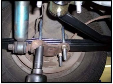
3. Loosen the lower shock nut allowing the plate to pivot.
