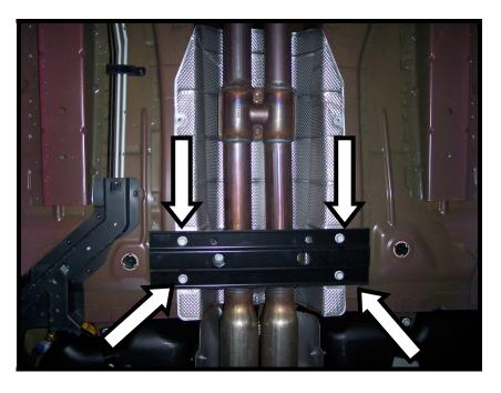
2. Install either side of the under brace by first placing the center mounting bracket holes where the stock plate was removed from. Use the stock bolts and the included LARGE washers for this bracket.
