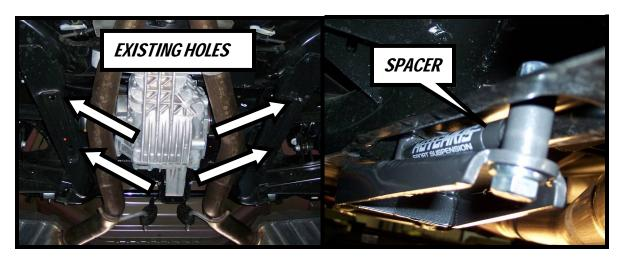
4. The Front bracket should now line up with its hole. Use the provided hex bolt and LARGE washer on that bracket.
