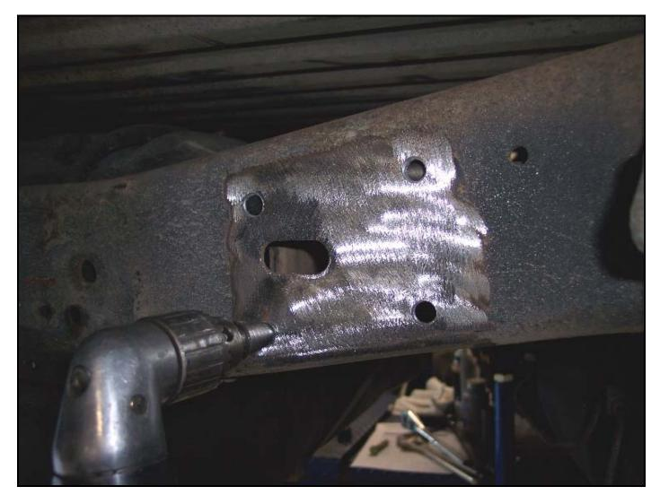
Once the holes are drilled, use the provided 3/8" hardware to mount the passenger side bracket to the frame. Fully tighten this hardware and the driver side hardware.
