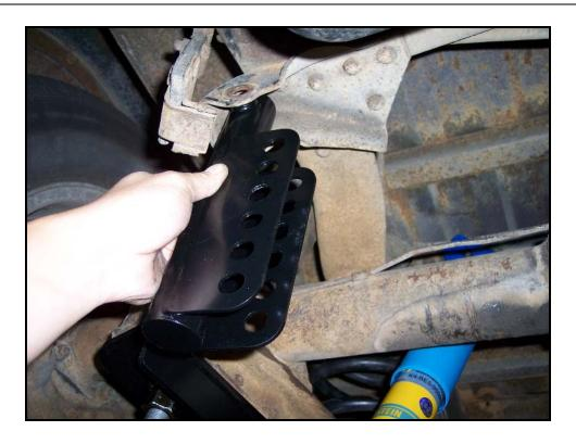
Take the  $\underline{\text{shorter}}$  adjustable bar and install it on the  $2^{\text{nd}}$  or  $3^{\text{rd}}$  hole on the driver side mount bracket. Grease bushing surface with provided lube.
