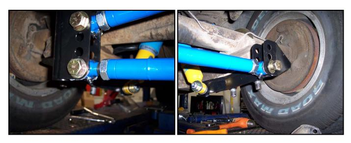
Once all of the suspension members are in place, measure the distance between the inside of the rear tires and the wheel wells. Adjust the track bar (lower one) in or out to equalize the tire gap. Once adjusted, fully tighten all of the hardware.
