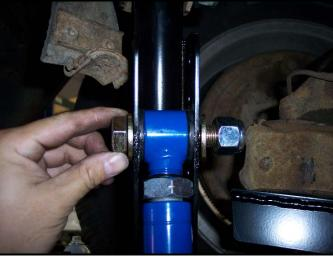
Attach the passenger side frame bracket to the bar using the included hardware.
