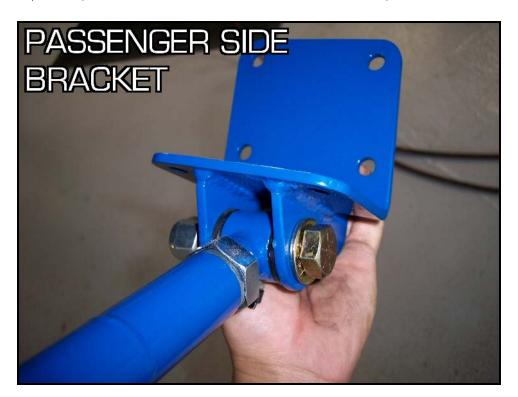
Adjust the length of the support bar so that the driver side bracket is <u>vertical</u> and the passenger side bracket mates to the frame rail properly.
