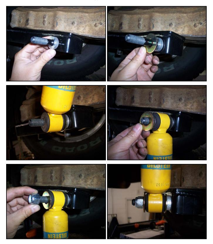
New hardware is also provided for the upper mount. The Hotchkis upper mount has 2 adjustment holes. The hole toward the rear is the stiffer shock setting. Once the shock is in place, fully tighten all shock hardware.
