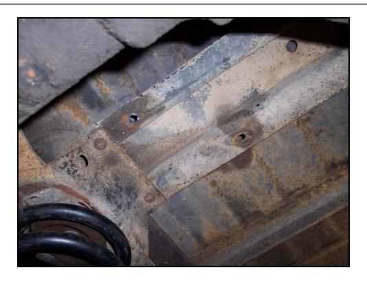
Next, remove the lower shock mounts by undoing the large u-bolts holding the rear axle to the trailing arms. The lower mounts should be loose from the arms. You may discard the upper and lower mounts.
