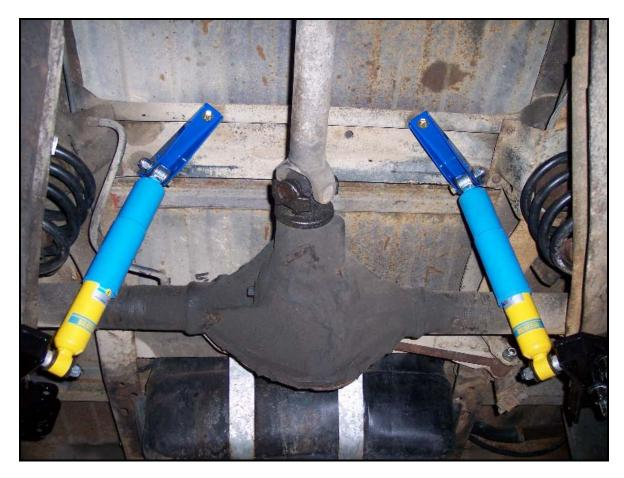
Lower the lifting jack from the trailing arms and you are now finished with the rear shock installation.
