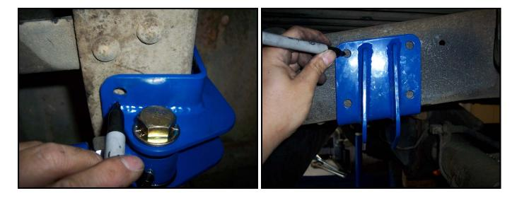
(Important Note: Make sure the bracket is not too far towards the rear, which may cause the rearward bolts to interfere with the frame support. Frame support held in by rivets shown in above pictures.)
