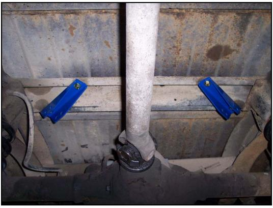
Install the lower shock mounts in the same manner as stock removal. Please see picture for proper orientation and placement of side specific brackets. Secure the lower shock mounts using the original u-bolt hardware. (Please call Hotchkis if you would like to purchase new U-bolts  $\rightarrow$  P/N: T1734) Fully tighten hardware at this time. (Tip: It is recommended that you apply anti-seize compound on the U-bolt threads before reinstalling the nut.)
