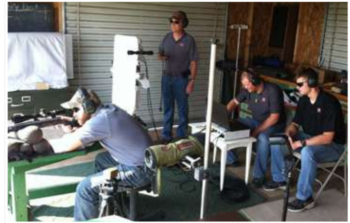
Hornady engineers used Doppler radar to discover the effects of aerodynamic heating and confirm the effectiveness of the Heat Shield® tip.
