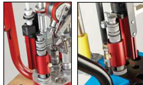
The case-activated Rifle Bullet Feeder is also compatible with the Dillon model XL 650.
