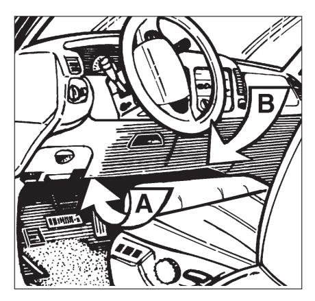
The location of the vehicle connector for 1994-98 F-Series Pickups can be found at the arrow marked "B". All other applications listed can be located at the arrow marked "A".
