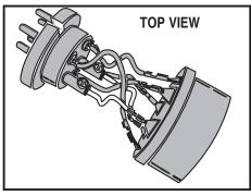
To change wiring functions, remove screws and switch blue & black wires.
