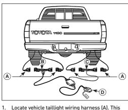
Locate vehicle taillight wiring harness (A). This
