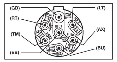
Loosen the set screw (A) and remove the terminal assembly (B) from housing. Route wiring through housing. Strip wires 1/4" and tightly secure them to the terminal assembly. It is important to attach wires to the terminal assembly in the same positions as found on the vehicle side 7-way socket. Leave 18" of slack between tow vehicle and trailer to allow trailer to turn. Align terminal assembly keyway (C) with housing key and insert assembly into housing. Tighten set server.
