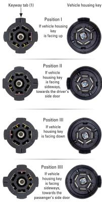
Once aligned properly, insert assembly into housing. Tighten set screws.
