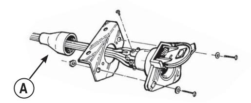
Loosen the set screw (A) on the connector and remove the socket from the housing. Route wiring through socket housing. Strip wires 1/4" and tightly secure them to socket terminals. Align socket keyway with housing key and insert socket into housing. Tighten set screws. Locate wires on vehicle by function only. Color coding is not standard with all manufacturers.
