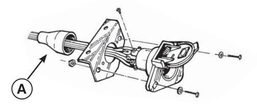
1. Remove rubber boot (A) from connector. Insert wires through the rubber boot. Strip 1/4" from wire ends and tightly secure them to the connector terminals. Replace rubber boot over terminal assembly.
