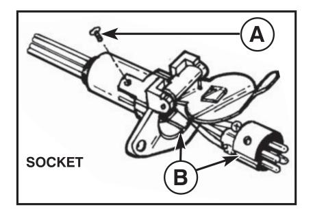
1. Loosen the set (A) screwon the vehicle end socket and remove the socket from housing. Route wiring provided through socket housing. Strip wires 1/4" and tightly secure them tosocket terminals. Align socket keyway (B) with housing key and insert socket into housing. Tighten set screw
