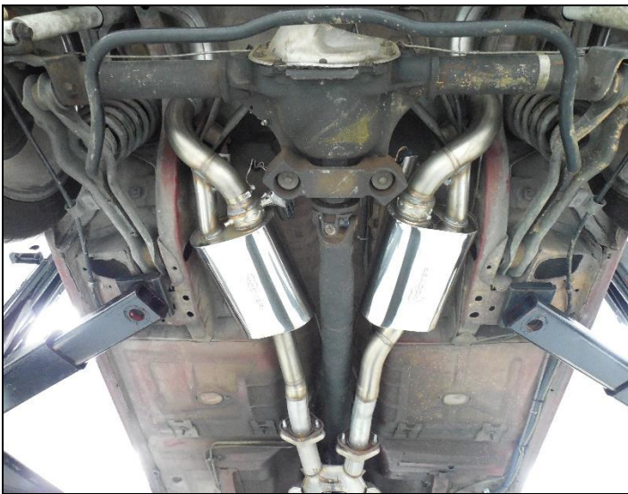
Figure 3 – Mid mount install w/ tailpipes
