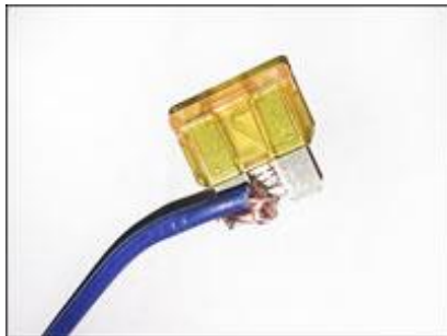
Wire Jammed Into a Fuse
