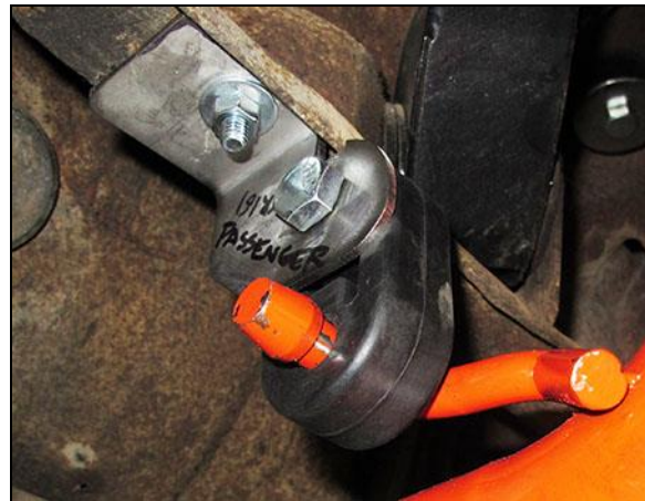
Figure 2 – Right over-axle hanger bracket
