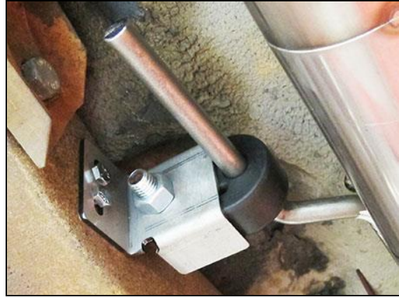
Figure 4 – Right tailpipe hanger bracket
