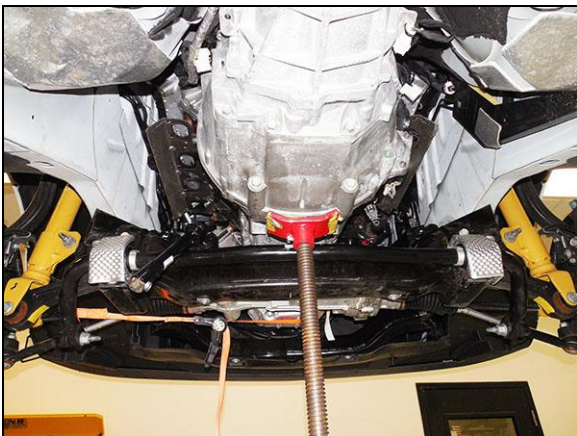
Figure 3 – Engine support and tie strap
