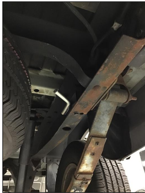
Figure 2 Rear tailpipe hanger to frame
