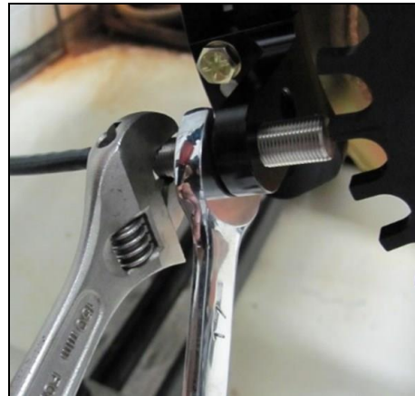
Figure 9: Locking the sensor gap.
