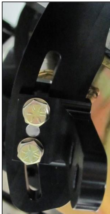
Figure 2: Centering the sensor bracket.
