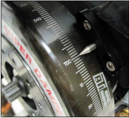
Figure 5: Rotating the engine to TDC #1.
