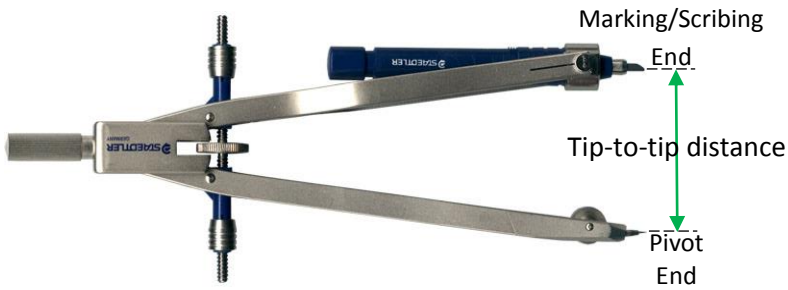
Figure 6: Drafting compass anatomy & tip-to-tip distance.
