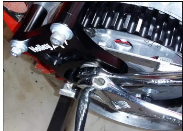
Figure 15: Locking Sensor Gap & Position
