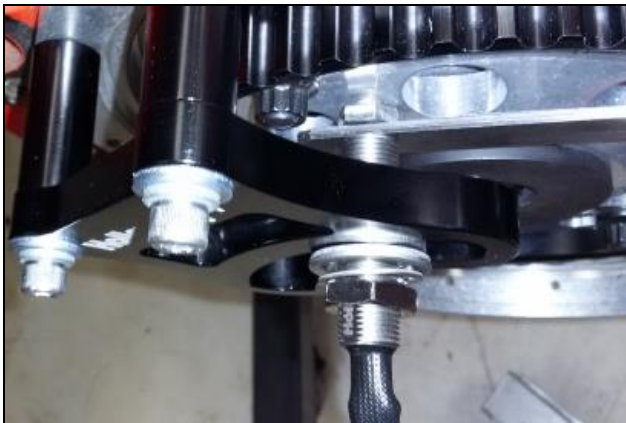
Figure 14: Adjusting Sensor Gap
