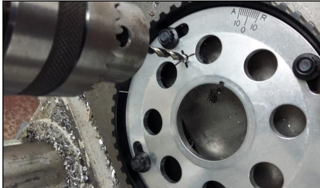
Figure 11: Drilling the Cam Hub.
