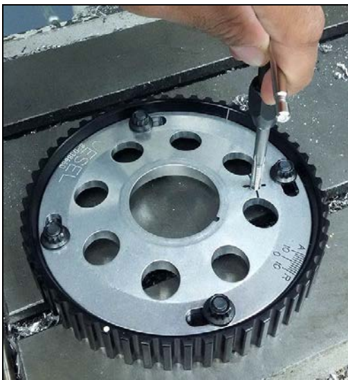
Figure 12: Tapping the Cam Hub
