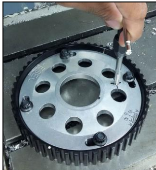
Figure 8: Tapping the Cam Hub
