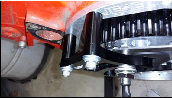
Figure 10: Adjusting Sensor Gap
