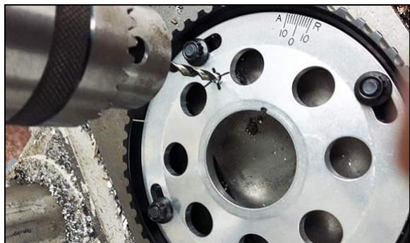
Figure 7: Drilling the Cam Hub
