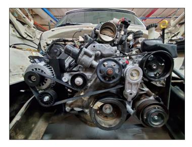
7. Attach all electrical connections to the alternator and start the engine. Observe the belt and ensure no slipping, binding, or excessive vibration is present.
