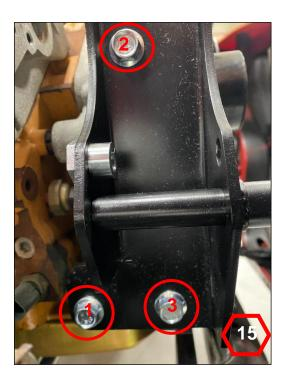
4. Next, slide the Holley alternator into place between the bushings and bracket. Torque the supplied M10 x 1.5mm x 80mm bolts to 36 ft./lbs. **NOTE:** A wrench may be needed to keep the bushings from rotating.
