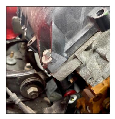
**3.** Clean the alternator mounting surface so that it is smooth and free of corrosion. Using the supplied M10 x 1.5 x 25mm bolts, install the alternator bracket following the sequence below. Torque each M10 bolt to 48 ft./lbs. (65N-m).
