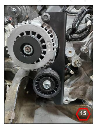
6. Inspect the assembly and ensure all hardware has been torqued to the proper specification. A longer belt is required since the alternator position has moved. Holley recommends using a **6PK2250**. This belt can be found at most automotive parts retailers. Below is the proper belt routing.
