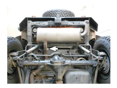
4. Remove nuts from stock and Flowmaster clamps, apply anti-seize compound to bolts and re-install nuts.
