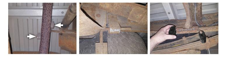
5. Remove clamp on muffler inlet, then remove muffler and set aside.
