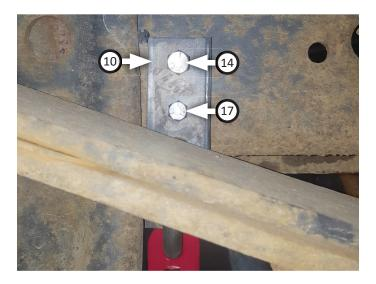
**NOTE:** If you have an aftermarket tow hitch (such as Drawtite), we have included a **bolt (21)** that will allow you to fasten **rubber hanger (13)** directly to side of tow hitch. There are (x2) holes located on side of hitch where mounting arms narrow toward front of vehicle. Place **rubber hanger (16)** up to forward hole and insert bolt with **flat washer (22)** through rubber hanger from inside of hitch.
