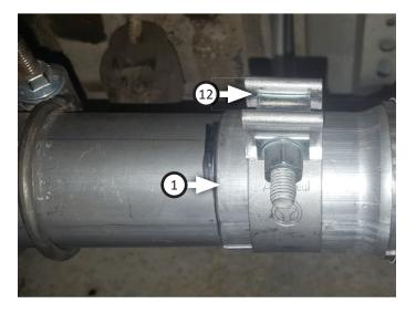
12. Place (x2) **clamps (11)** onto **muffler (3)** and connect it to adapter pipe. Tighten front clamp just enough to allow for adjustment.
