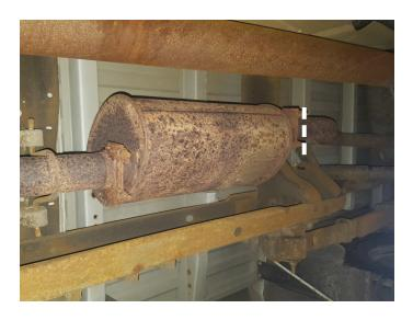
4. Separate wire hangers from isolators behind muffler. Remove bolt and hanger connecting stock tailpipe to vehicle frame. Remove tailpipe section from vehicle.
