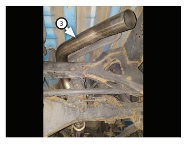
10. Place **clamp (5)** onto **exit pipe (4)** then connect it to over-axle pipe. Insert wire hanger into rubber hanger then tighten clamp just enough to allow for later adjustment.
