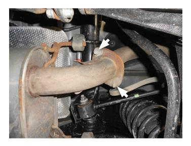
Remove bolts from front flange connection and retain (x2) springs for later use. Separate wire hangers from isolators and remove muffler assembly from vehicle.
