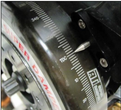
Figure 1: Rotating the engine to TDC #1.
