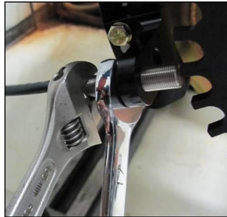
Figure 4: Locking the sensor gap.
