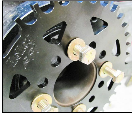
Figure 7: Fastening the Crank Wheel to the Balancer
