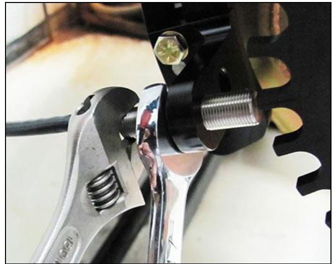
Figure 9: Locking the Sensor Gap
