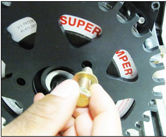
Figure 7: Fastening the Crank Wheel to the Balancer
