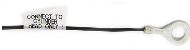
Figure 22 Coil Ground Wires
