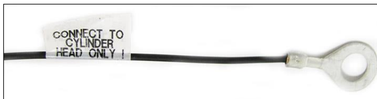
Figure 26 Coil Ground Wires
